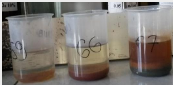
After oxidation with 60 mg/l of ferrate
