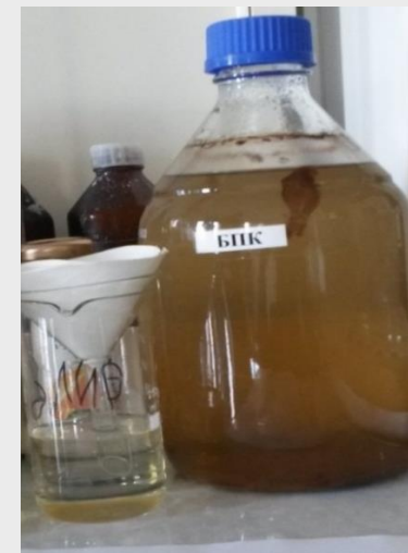
Sewage before (to the right) and after the oxidation with 15 mg/l of ferrate
